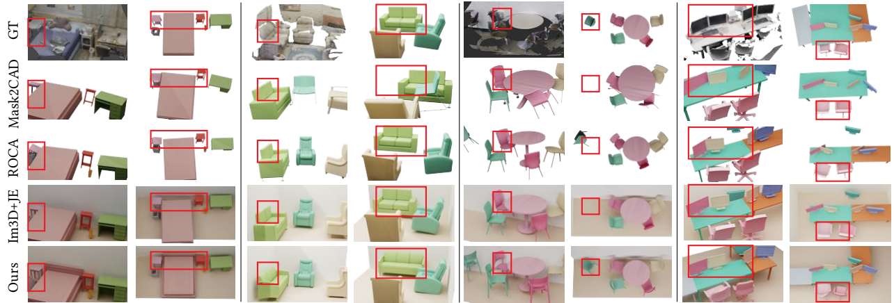
Fig. 1. Qualitative comparisons with single-frame baselines, including Mask2CAD [Kuo et al. 2020], ROCA [Gümeli et al. 2021], the combination of Im3D [Zhang et al. 2021] and Joint-Embedding [Dahnert et al. 2019] (Im3D+JE) and our method. The top left image of each group is the input for each method, and the top right one is the corresponding GT reconstruction result of the input.
